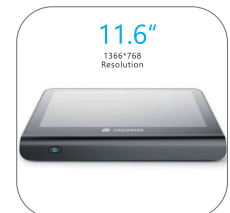
11.6 inch TFT LED Backlight Projective Capacitive Touch Screen
