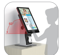
Ergonomic design, 60° tilted display stand provides comfortable operation and perfect viewing
